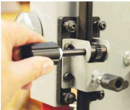
The depth of cut is altered with this heavy-duty rack and pinion setup
